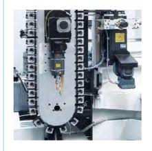
Versatile: disc magazine with two independent magazine discs enables extremely fast provision of up to 120 tools.
